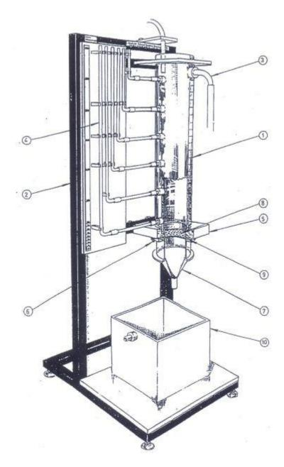
Figure: Drain Permeator
