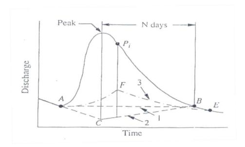
Fig.4: Base flow separation methods
