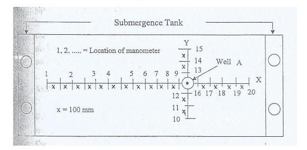
Figure.2: Locations of manometer tapping and wells
